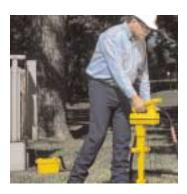
**Tailored to Meet Your Needs.**The new 3M Dynatel 2200M Series Locators offer several features for cable/pipe locating with more accuracy, speed and sensitivity than ever. These receivers provide two directional modes: Directional Peak and Directional Null; plus an ultra-sensitive Single Peak mode for extreme depths. They also incorporate an "expander" function to make peaks and nulls more pronounced by enhancing the amplitude difference between two conductors carrying the same tone.
